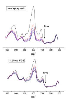
Figure 1b: Real-time FTIR conversion curves as a function of irradiation time for the pristine CE resin ( $\square$ ) and for the epoxy resin formulations containing 0.5 ( $\circ$ ), 1 ( $\bot$ ) and 1.5 ( $\top$ ) wt% of the graphene. Light intensity on the surface of the sample 35mW/cm<sup>2</sup>. Film thickness 25  $\mu$ m.
